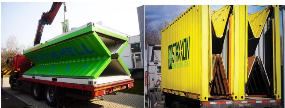
Figure 3-46: Folding shipping container concepts
